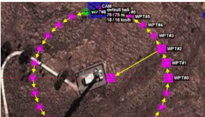
Picture 2: Pre-programmed waypoints of the helicopter's flight route
