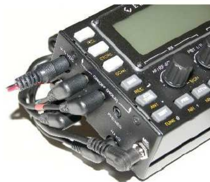
Figure 2 — The side panel of the KX3 is the location of all the external interconnection points, except for the antenna. By using the optional KX3-PCKT Accessory Cable Set, all the connections except the power cable terminate in right angle plugs allowing neat routing of the accessory cables.
