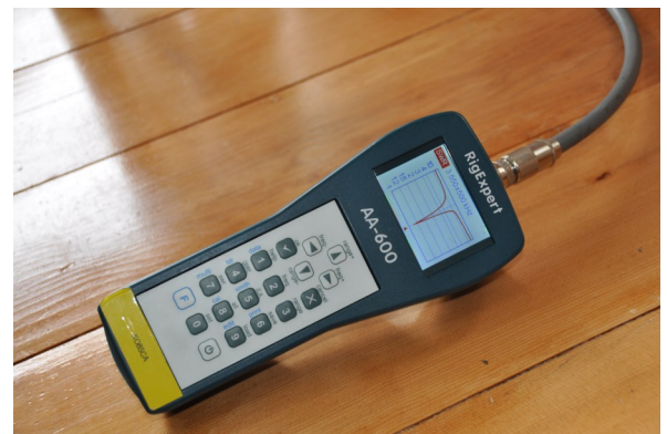
The RigExpert AA-600 antenna analyzer helped tremendously in tuning the new 80M rotating dipole
