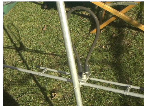
Fig 32 – A Half-Wave Balun
