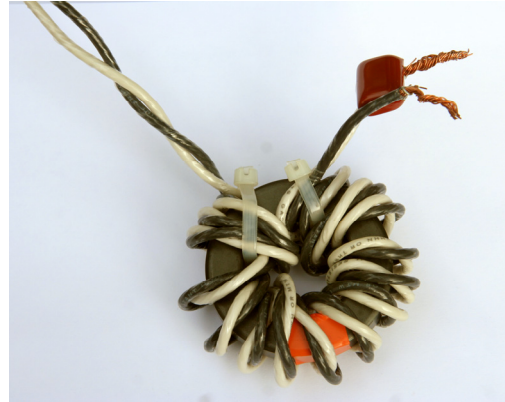
Fig 30 – A line filter for 1-14 MHz
