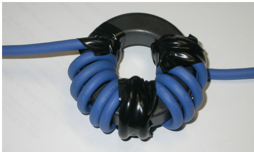
Fig 4 – A toroidal ferrite choke
