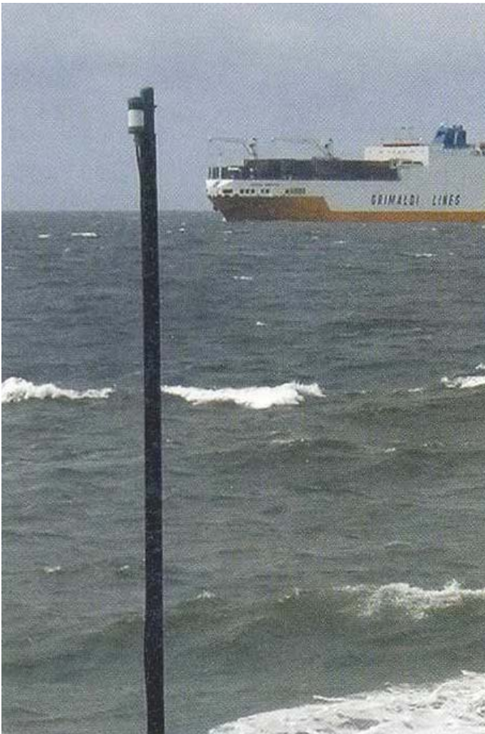
Photo 8 - Westkapelle, the Mini-Whip on a plastic mast section.
