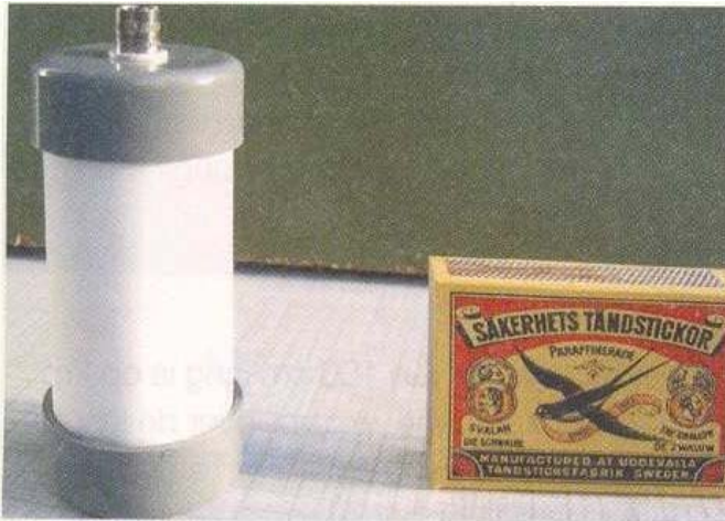
Photo 3 - Standard form of pa0rdt-Mini-Whip ©.
