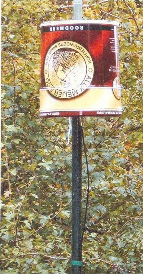
Photo 6 - Passive E-field antenna.
