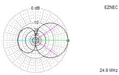
Azimuth Plot Elevation Angle 0.0 deg. Outer Ring 5.48dBi Cursor Az 0.0 deg. Gain 5.48 dBi 0.0 dBmax
