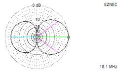
Azimuth Plot Elevation Angle 0.0 deg. Outer Ring 3.74dBi Cursor Az 0.0 deg. Gain 3.74 dBi 0.0 dBmax
