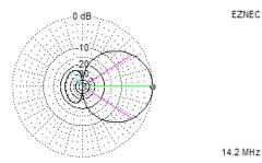
Azimuth Plot Elevation Angle 0.0 deg. Outer Ring 7.36dBi Cursor Az 0.0 deg. Gain 7.36 dBi 0.0 dBmax
